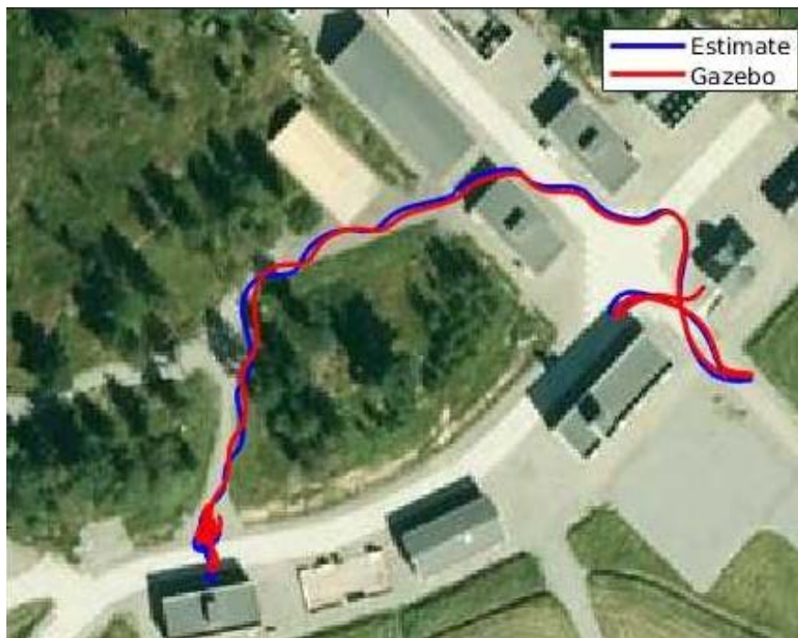
Figure 1: Actual (red) and estimated (blue) UAV trajectories during a simulated flight, overlaid on the reference image used for navigation.
